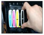
Remove the original cartridges
