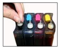
Place 4pcs of air filters into air holes, the thicker side is down into tank.
